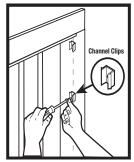
drill bit) and install the channel clips, using five of the 1" roundhead screws. Align the clips vertically and press the door anchor panel onto them until it snaps into place.
