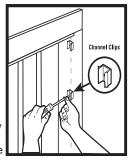
or a 3/32" drill bit) and install the channel clips loosely, using five of the 1" roundhead screws. Align the clips vertically and fully secure the screws. Press the door anchor panel onto them until it snaps into place.
