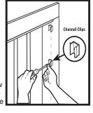
or a 3/32" drill bit) and install the channel clips loosely, using six of the 1" roundhead screws. Align the clips vertically and fully secure the screws. Press the door anchor panel onto them until it snaps into place.
