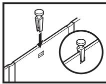
To secure the T-style lead edge top glide, place the T shaped part inside the lead edge and align the holes. Then insert the female section from the outside hole through the hole in the T shaped glide through the other side of the lead edge. Then insert the threaded male screw into the female part and tighten until snug.
